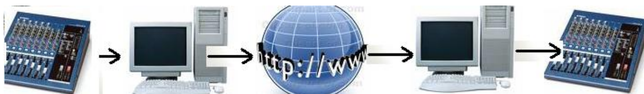
1. OB mixing panel ... to...2. OB Computer...to...3.Internet as a continuous stream... to...4. Studio Computer...to...5... Studio mixer
